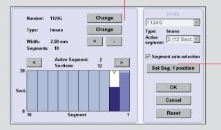
To optimize diamond knife usage, up to 100 different knives can be stored. Each knife is divided into a number of segments. The selected segment is approached automatically with the motorized knife stage (patent applied).
