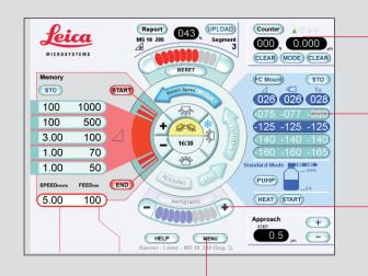
Counter window to toggle between section counter and feed totalizer, countdown, E-W measuring, and AutoTrim mode.
