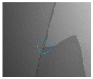
Cross section of a tooth with inlay (filling) prepared with the Leica EM TXP (area of interest marked blue).
