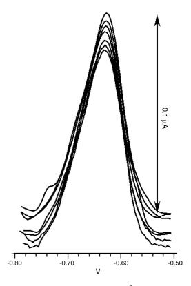
Fig. 4. Reproducibility of the signals of 10 ppb Pb<sup>2+</sup> from seven consecutive measurements, 2-min preconcentration period, other conditions as in Table 1.
