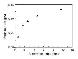
Fig. 2. Effect of preconcentration time (adsorption at open circuit) on the signals of 10 ppb  $Pb^{2+}$ , operating conditions as in Table 1.
