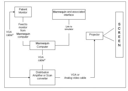
+ VGA cable source and routing will vary depending on mannequin manufacturer. Several different lavouts are represented here
