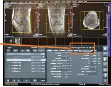
The first two numbers are the *pixel size* followed by the *slice thickness*. In the example above the reconstructed pixel size is 0.51x51 mm and the slice thickness is 0.51 mm.
