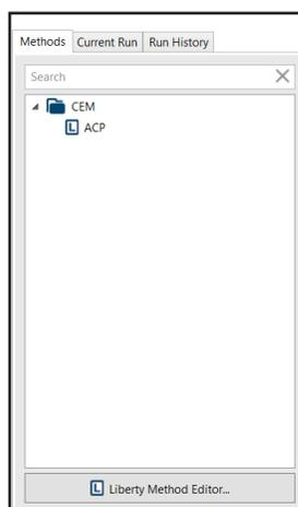
**Methods:** From this tab, methods are loaded into the resin position.
